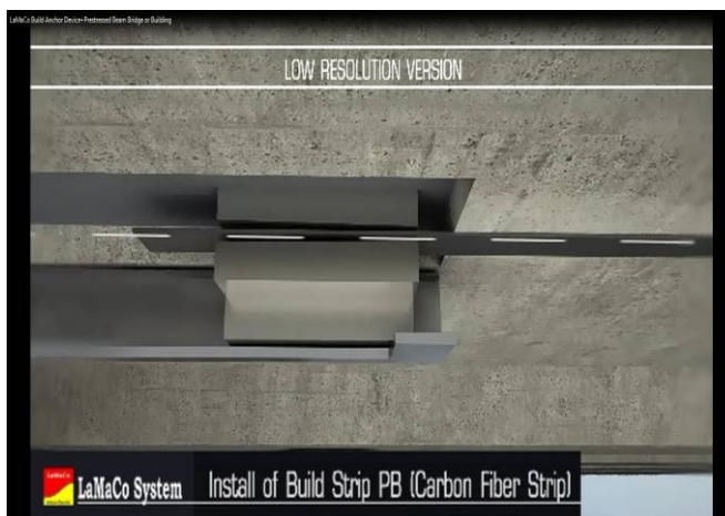
11] Install the Build Strip PB in Position
